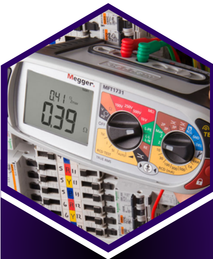
Testing LV & control cables, including meggering and loop test
